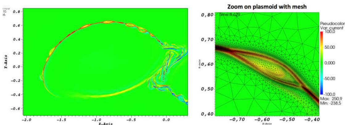
**Figure 1:** A current layer with a plasmoid chain (left). Zoom on a single plasmoid overlaid with mesh (right).
