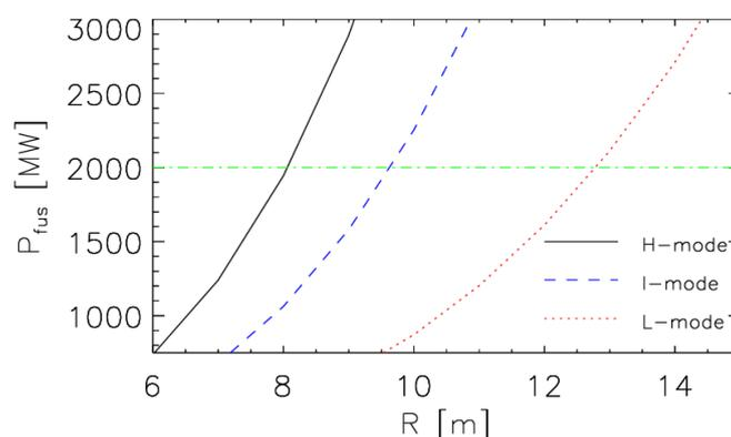
**Figure 1:** Fusion power as a function of size of the machine for  $H$ -,  $I$ -,  $L$ -mode. The quantities in common to the regimes considered for the plot are  $B = 6$  T,  $q_{95} = 3.5$ ,  $A = 3$ ,  $P_{aux} = 50$  MW and  $P_{rad} = 200$  MW.
