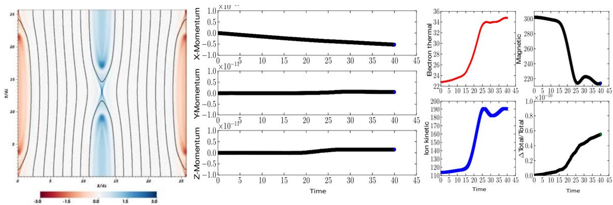
**Figure 1:** Left: Current density  $j_z$  and contours of the magnetic potential  $A_z$  for the GEM Challenge reconnection problem [2]. Middle: Momentum errors in each direction vs time, demonstrating strict momentum conservation. Right: Traces of the electron thermal energy, magnetic energy, ion kinetic energy and the relative total energy error vs time, demonstrating strict conservation of energy.
