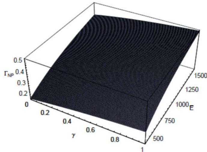
**Figure 1:** The surface plot of the fusion penetration factor  $\Gamma_{NP}$  in nonideal plasmas as a function of the nonideality parameter  $\gamma$  and the scaled energy of the reactive motion  $\bar{E}$  when  $\bar{\lambda}_D = 10$ .
