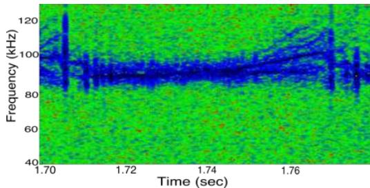
**Figure 1:** Frequency spectrogram for AUG discharge 20488 from  $t = 1.72$  to  $1.78$  seconds. Strong BAE mode activity during monster saw-tooth crashes is measured with Mirnov coils.
