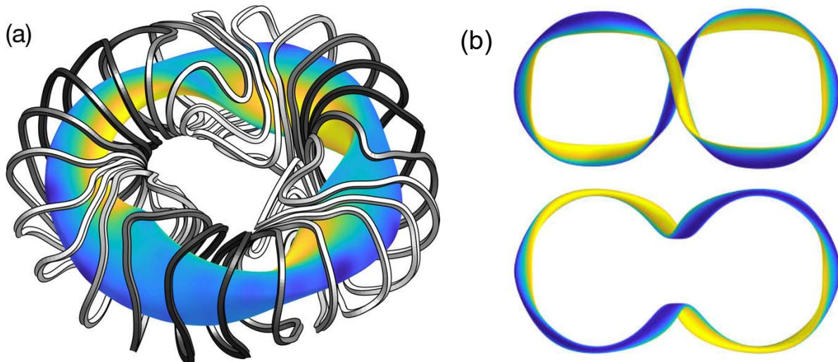
**Figure 1:** A (a) quasi-axisymmetric and (b) quasi-helically symmetric stellarator configuration generated by the direct geometric construction of [4]. Color indicates  $|B|$ .
