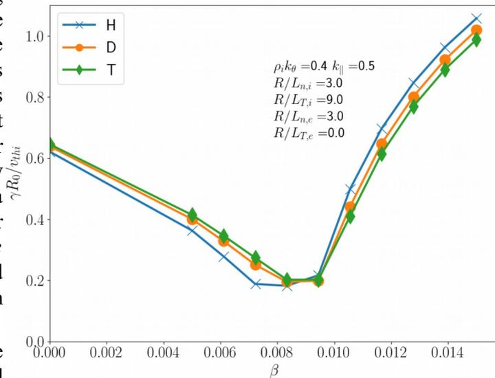
Figure 1: ITG growth rate as a function of the plasma beta  $\beta$  for the hydrogen (H), deuterium (D) and tritium (T). GKW simulations
